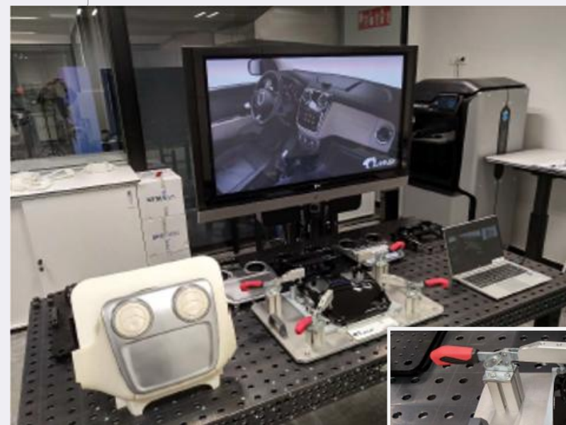
r-PC/ABS (VTT), 2K injection moulded dashboard console (ABA) MAIER
