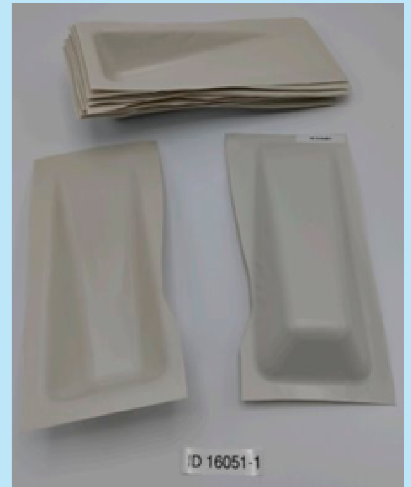
Figure 16. Thermoformed test samples containing 70% rHIPS (VTT). Compounding on VTT’s cascaded mechanical recycling line. The rHIPS flakes for the compounding were from dismantled refrigerators (Coolrec)
