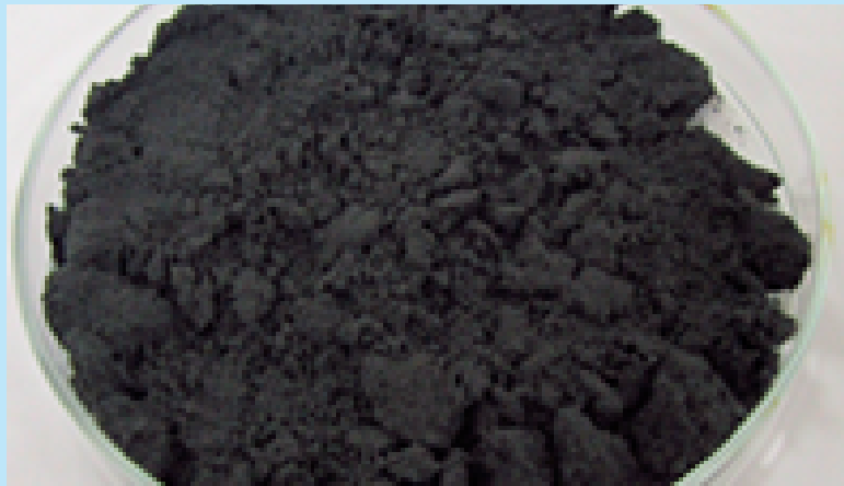
Figure 20. Recyclate produced by grinding the end of life washing machines
