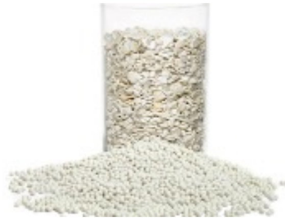
Figure 15 - rHIPS flakes (before extrusion) and granules (after extrusion).
