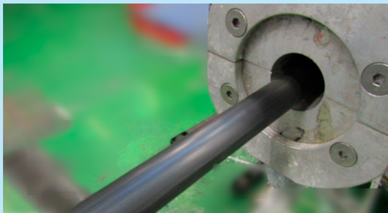
Figure 10. Extrusion of TPV material
