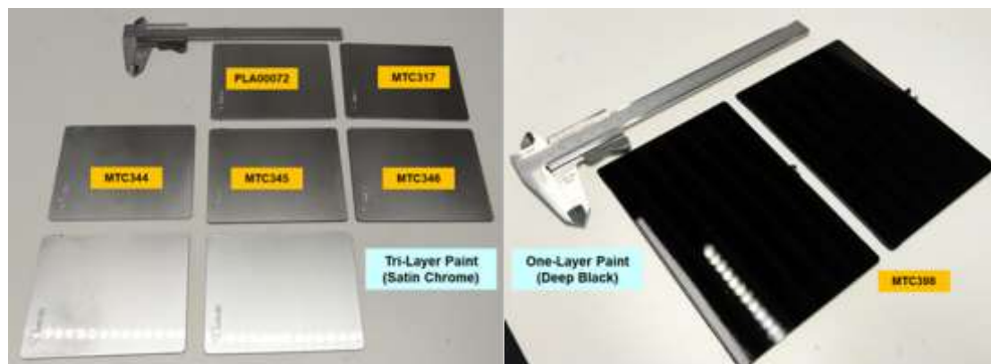
Figure 7. Painted sample parts. Tri-Layer Paint (left) and On-Layer Paint (right)
