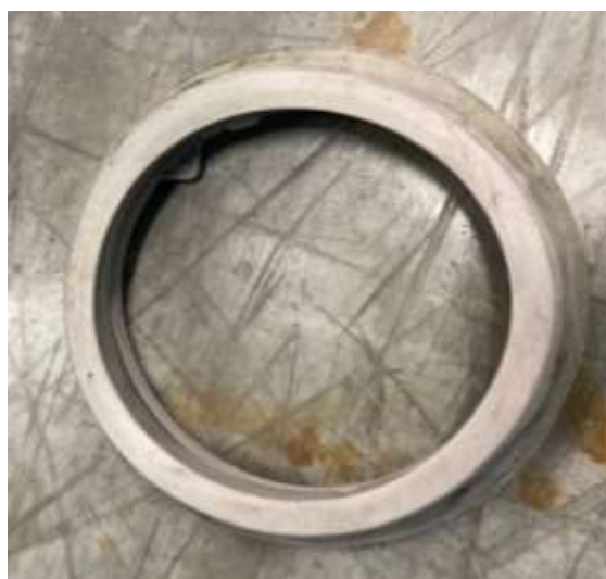
Figure 24. Example of a door gasket that has been discarded to produce dark grey gaskets due to its colour.
