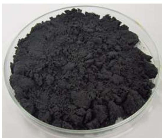
Figure 28. Micronised EPDM powder obtained by cutting end-of-life gaskets.
