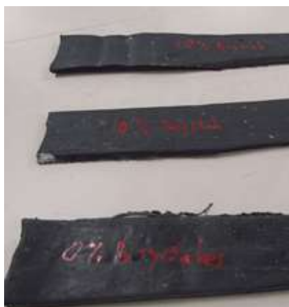
Figure 30. rubber compounds with 0%, 10% and 20% of recyclates.
