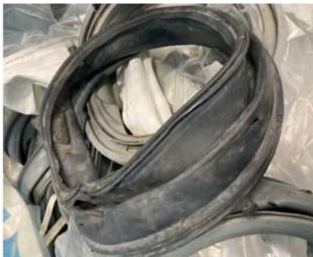
Figure 23. End-of-life washing machine door seals.
