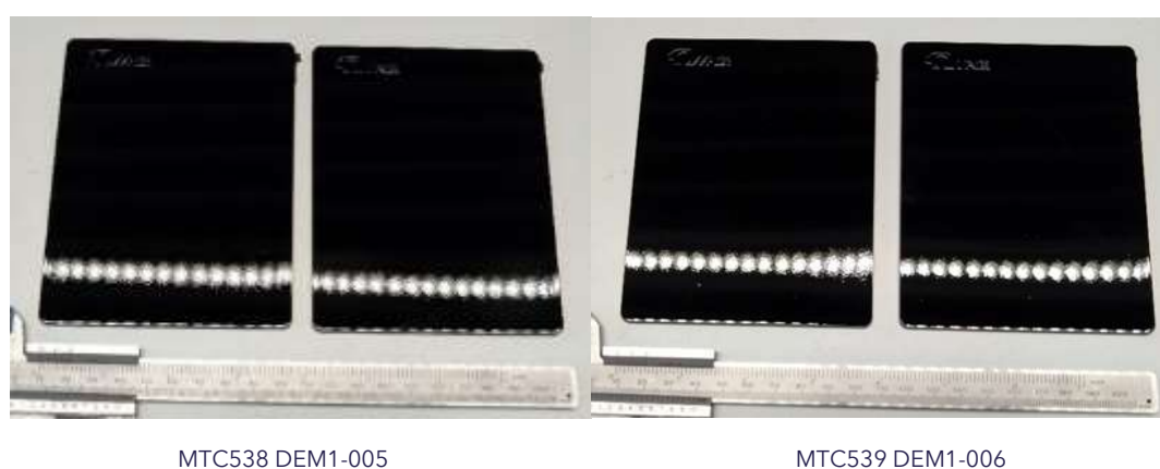
Figure 8. Painted sample parts. On-Layer Paint. r-PC/ABS prototype formulations.
